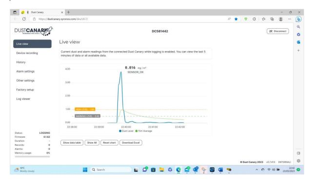
Dust levels shown on *Live View* may be downloaded as an Excel file via the Download Excel button. Note that the recorded data sessions in the device cannot be accessed with *Live View* and should instead be downloaded from the *Device Recording* and *History* tabs.
