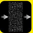
Removes particles > 4µm (allows respirable dust to pass)
