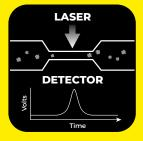
Counts and measures particles in predetermined particle size cuts
